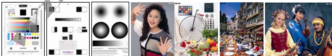
Image-quality originals used by Wirth Consulting when evaluating a device's image quality.
